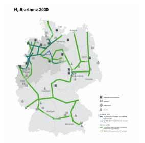
German Gas Transmission Network Operators have published a plan for a new nationwide hydrogen network to take hydrogen between sites of production (e.g. electrolysis near the coast where offshore wind is connected), sites of storage (underground caverns) and consumers of hydrogen (industry, etc.).
