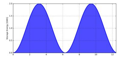
Although wind and solar are not perfect sine waves, if we decompose the time series in Fourier components, we do see **dominant frequencies** which can help us understand how to dimension storage.
