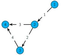
Focus on 3rd column of PTDF and look at power flow with  $p_3 = +1$  and slack  $p_1 = -1$ . Coefficients determined by resulting flow:
