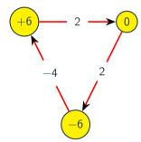
Along 2-edge path reactance is double the 1-edge path, so half as much power flows along the 2-edge path as the 1-edge path.
