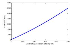
Note that the slope is always positive and becomes more positive for increasing g. The curve does not start at the origin because of startup costs, no load costs, etc.
