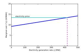
The area under the curve is generator costs, which as the integral of a derivative, just gives the cost function C(g) again, up to a constant.
