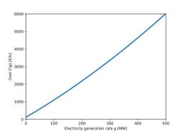
Note that the slope is always positive and becomes more positive for increasing g. The curve does not start at the origin because of startup costs, no load costs, etc.
