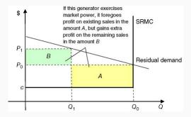
Generator will choose to produce at a lower rate of production if area B is larger than area A (depends on various factors).
