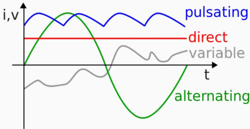
[Some power is transmitted as **Direct Current (DC)** under bodies of water Source: Wikipedia and indeed many electronic devices require DC (must convert AC to DC).]
